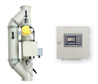
The Online Moisture Measuring Unit MC is used for continuous monitoring of moisture contents of free-flowing bulk solids, in particular grain and granulates. A high frequency probe, centrally mounted in a measuring pipe, measures the relative permittivity and temperature of the bulk material passing the probe. These values are continuously processed by the evaluation unit in order to determine the moisture contents of the material; this is then displayed digitally.
